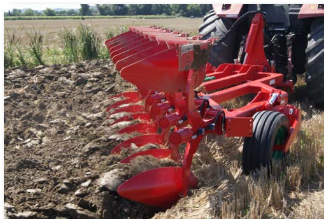
- Mini: el popular arado superficial de Ovlac para labores de hasta 20cm. - Mini: Ovlac's popular shallow ploughs to work up to 20cm deep.
