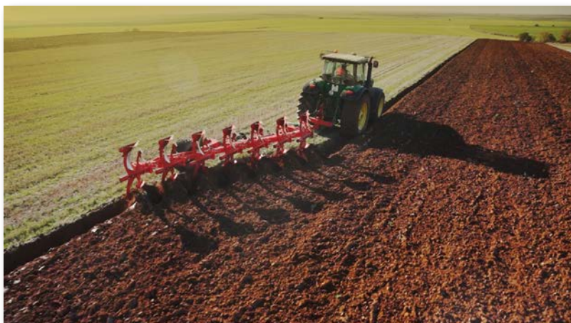
- Arados de vertedera de 3 a 9 cuerpos. Suspendidos y Semi-suspendidos. - Mouldboard ploughs from 3 up to 9 furrows. Mounted and semi-mounted.
