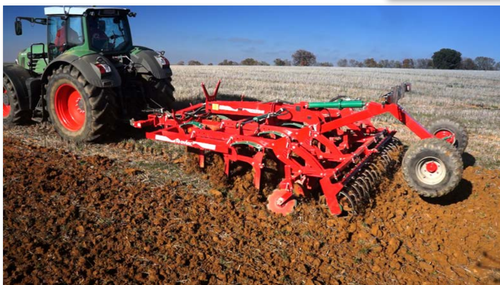
- Mini: el popular arado superficial de Ovlac para labores de hasta 20cm. - Mini: Ovlac's popular shallow ploughs to work up to 20cm deep.
